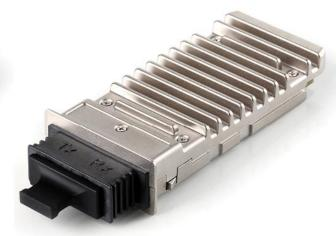
The X2-10GB-LR is a highly integrated, Serial optical transponder module for high-speed, 10Gbit/s data transmission applications. 4×3.125Gbps Ethernet Signal Input by XAUI Interface.An integrated Coder / Decoder and multiplexer / demultiplexer (SERDES: Serializer / Deserializer). Designing for 10km Transmission with an uncooled directly modulated 1310nm DFB Laser. Digital diagnostics
