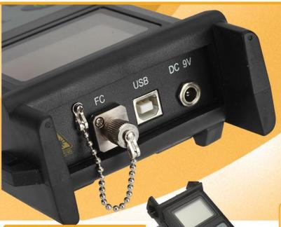
FO-TF4000 Optical fiber ranger is test equipment that functions similar to an optical time domainreflectometer. It is used in single mode fiber test applications. The fiber optic ranger is much smaller size and lighter weight compared to the fiber optic OTDR, and it is much more cost effective. They are used in optical fiber links trouble-shooting, maintenance and test.
